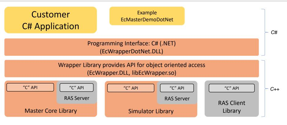
The example **EcMasterDemoDotNet** and the .NET wrapper are written in C#. The target platform is AnyCPU. The other libraries are written in C++ and are platform specific. The Wrapper Library is a helper that prepares the API for .NET. The demo runs in conjunction with Microsoft .NET framework.
