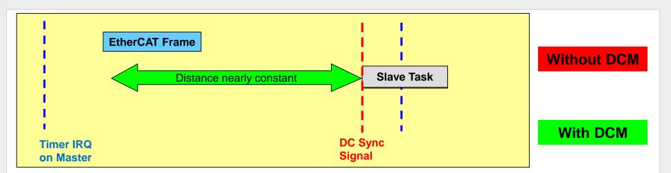
Blue line: Start of cyclic task (Job-Task) driven by oscillator on master controller
